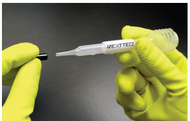
Figure 3 Allow Air to Enter Bellows
